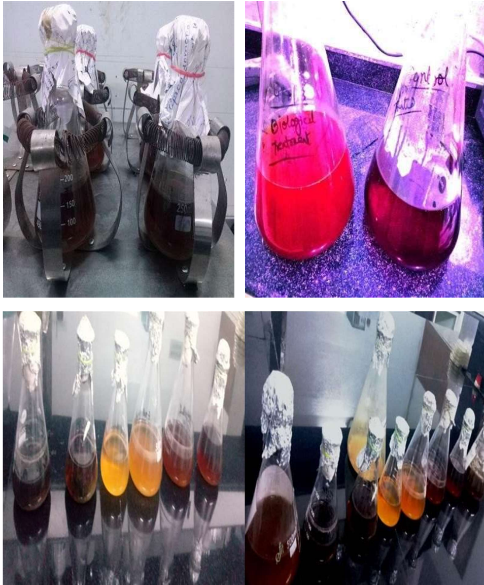
Figure 4.3 (b): Submerged (liquid) fermentation of iron oxidizing bacterial isolates
