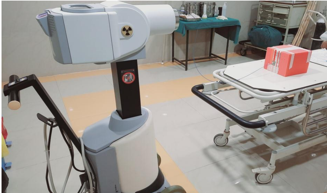
Figure 16: Showing a Phantom Connected to HDR machine for irradiation
