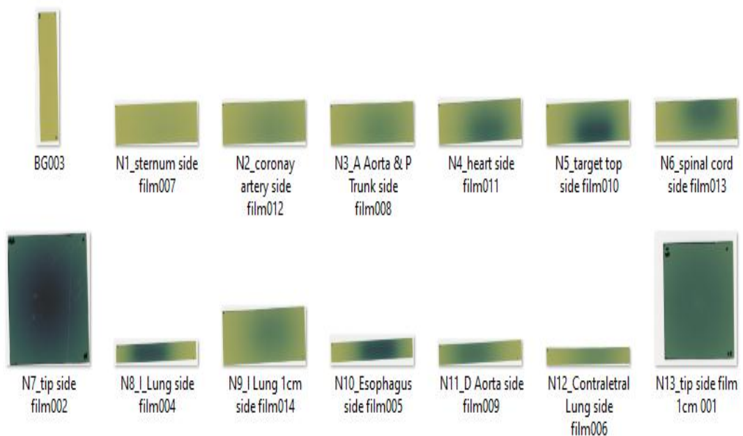
Figure 17: Showing the scan images of irradiated EBT3 films at different locations in the phantom.
