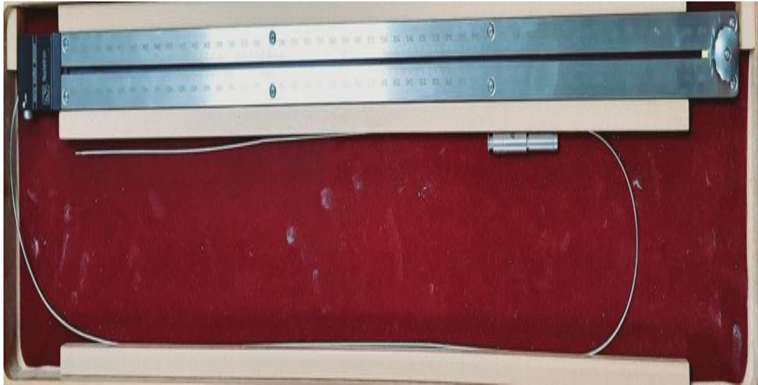
Figure 18: Showing a source position simulator tool at the time of CT scan
